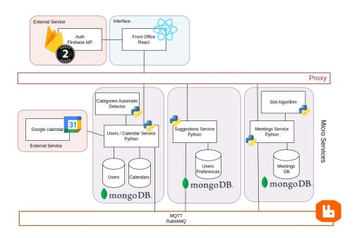
Figure 4.3: Final version of the architecture
